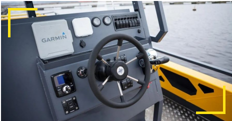
The helm console, wheel, engine controls and switch panel
