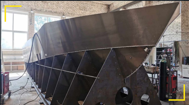
The hull on its jig, transverse frames and cut-outs along the length.
