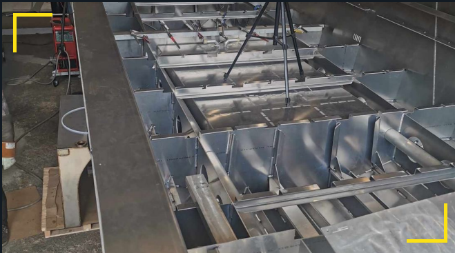
Looking down the hull at the welded frames and the buoyancy compartments.
